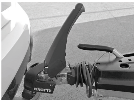
Fig. 9: Tow-ball coupling closed, stabilisation deactivated
