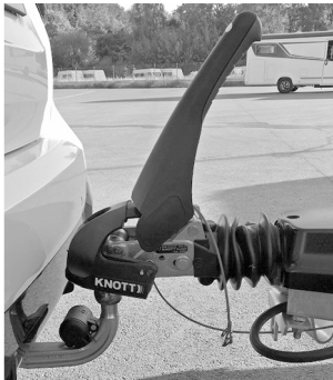
Fig. 13: Tow-ball coupling opened, stabilisation deactivated
