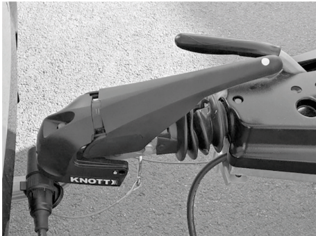
Fig. 10: Tow-ball coupling closed, stabilisation activated
