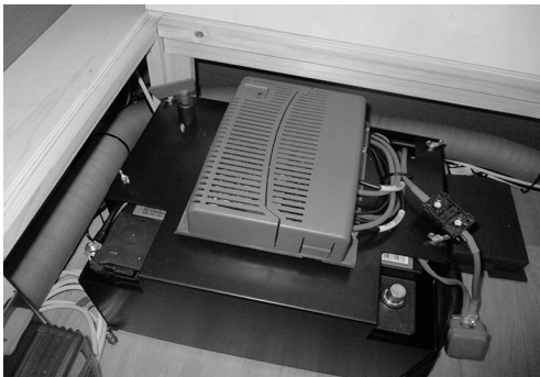
Fig. 77: Battery cover with control module for mover (optional)
