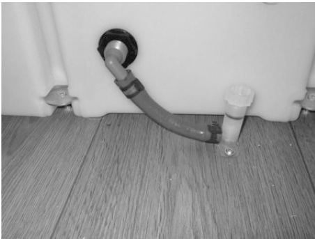
Fig. 90: Drain valve, example
