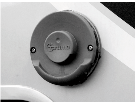
Fig. 81: Wall exhaust stack
