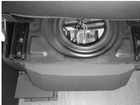
Fig. 8: Interface module under the driver's seat
