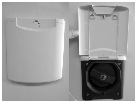
Fig. 86: Fresh water intake port
