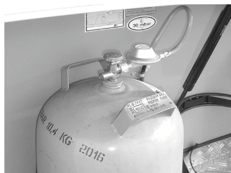
Fig. 63: Gas bottle with low pressure regulator and low pressure hose
