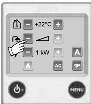
Fig. 141: No hot water
