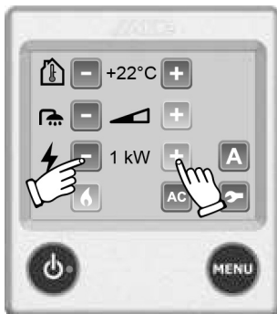
Fig. 145: Heating with electricity
