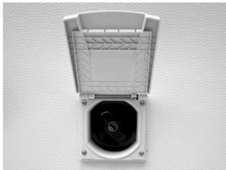
Fig. 93: Fresh water intake port
