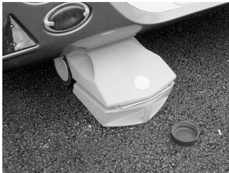
Fig. 110: Wheeled waste water tank
