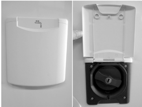
Fig. 102: Fresh water intake port
