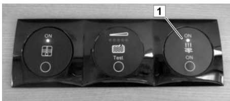
Fig. 92: On-Off switch of the floor heating system
