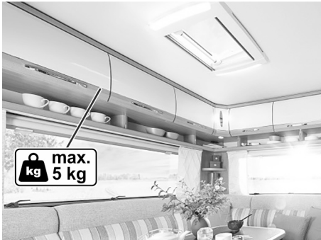
Fig. 56: Wall cupboards in the living area
