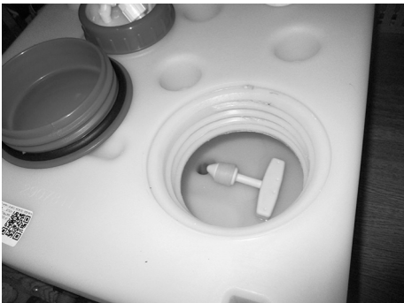
Fig. 105: Drain plug in the fresh water tank
