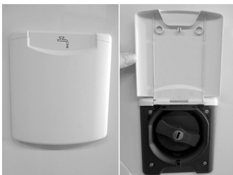
Fig. 27: Fresh water intake port
