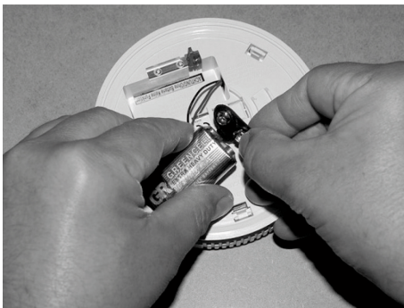
Fig. 161: Replacing the block battery
