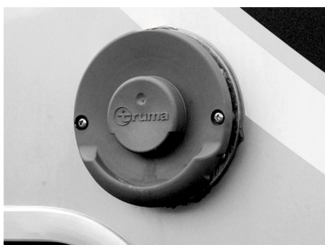
Fig. 74: Wall exhaust stack
